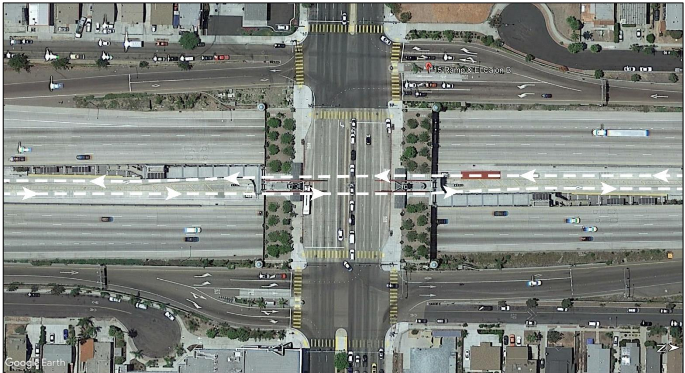
Figure 16 Aerial View of Split Platform Station at I-15 and El Cajon Boulevard
