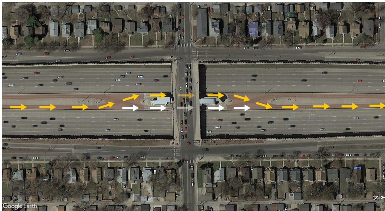
Figure 11 Aerial View of Median Crossover Platform Station for Part-time Shoulder Use at I-35W/46th Street
