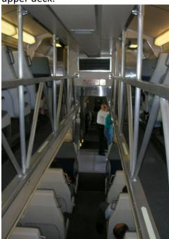
"Bombardier" cars with dual door entrances at opposite ends and 2+2 seating on both the upper and lower decks.
