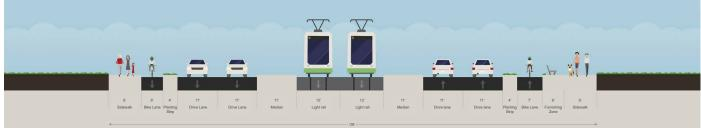
lanting strips separating the bike lanes function as rain gardens and would collect surface run-off.
