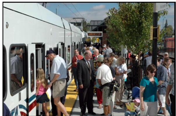
Low Floor Vehicles Provide Level Passenger Boarding
