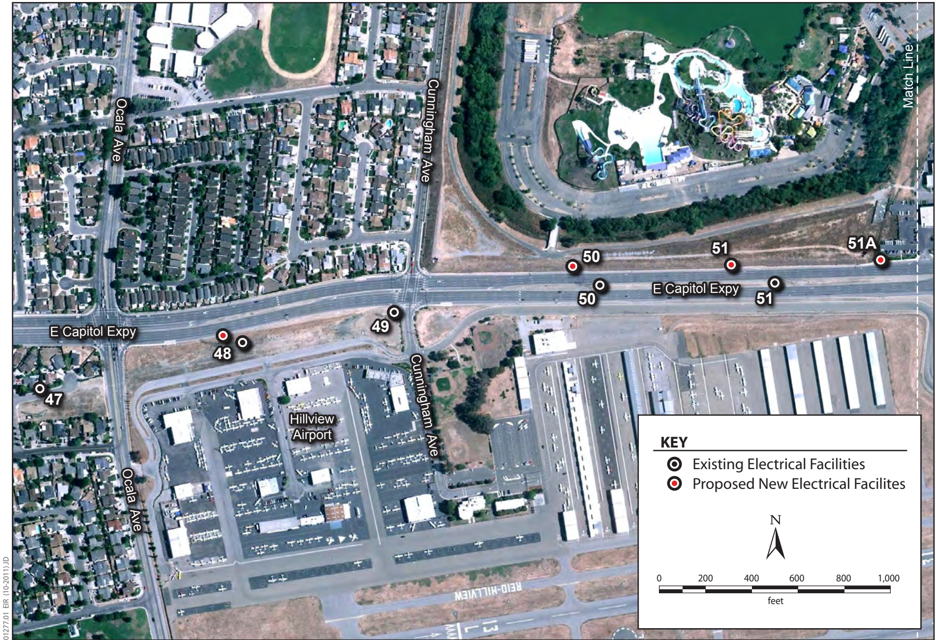
Figure 3.15-2a Proposed Changes to Electrical Transmission Facilities
