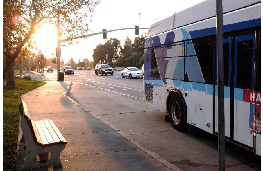
The Line 25 bus has many bus pullouts on the corridor today, requiring the bus to merge into and out of traffic, a common source of delay.
