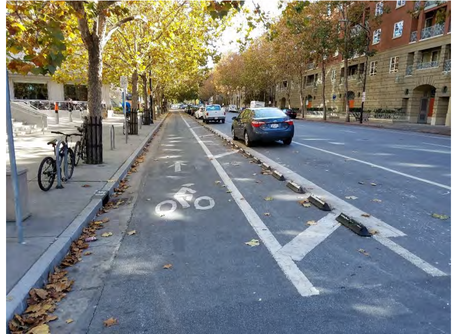
Example of a parking-separated bikeway with a buffer providing for loading and unloading.
