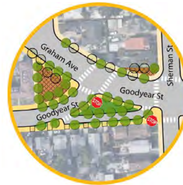
Top Left and Right: Roundabouts are the preferred improvements at Willow Street/Lick Avenue and Willow Street/Graham Avenue. At Goodyear Street/Graham Avenue, squaring up the intersection is proposed (at left).
