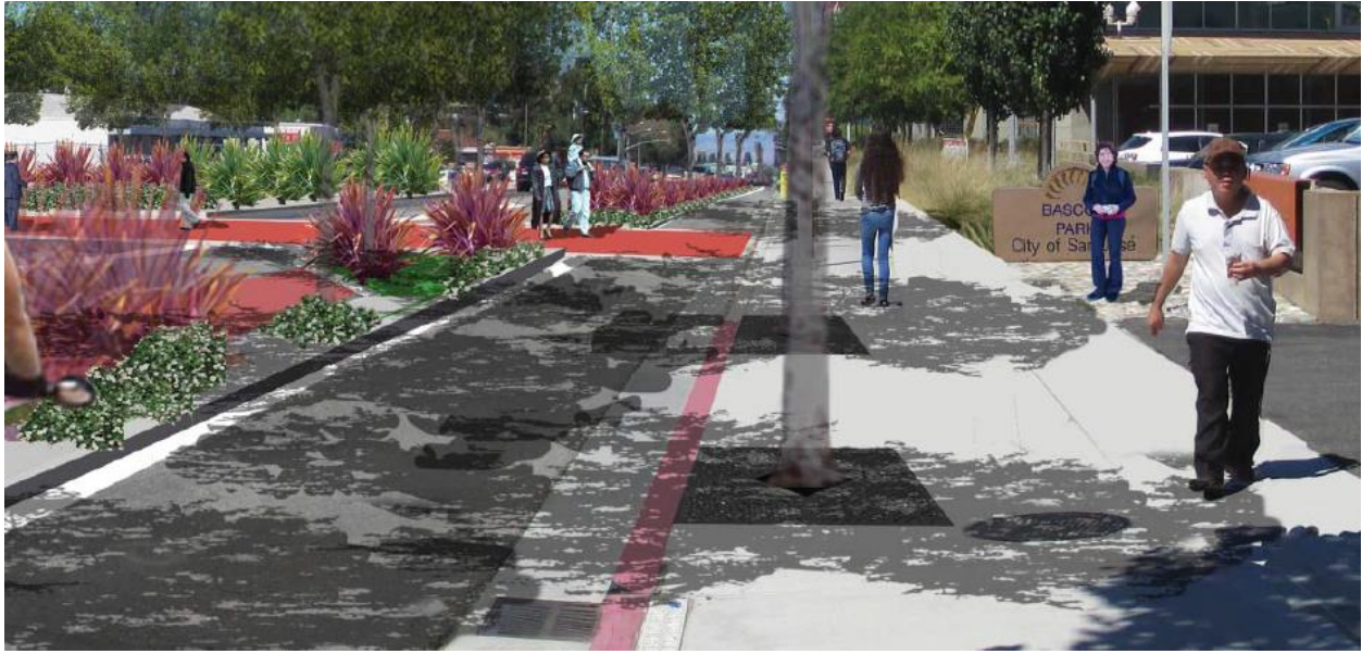
Figure 16. Photosimulation showing wider sidewalks, improved crosswalks, shade trees, & a cycle track with a planted buffer
