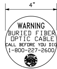
PERMANENT FIBER OPTIC CABLE MARKER (PAVED AREA)
