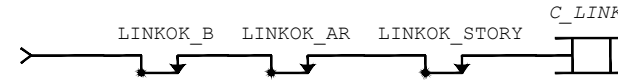
Link Health Status Central Office Indication Note: LINKOK_B - Link Health Status to "B" Electrologixs LINKOK_AR - Link Health Status to Alum Rock Electrologixs LINKOK_STORY - Link Health Status to Story Station Electrologixs
