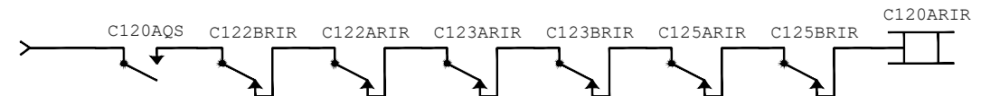
Route Initiation Circuit, Signal C120 "A" Route - to Signal C125 (Normal Running to Eastridge)
