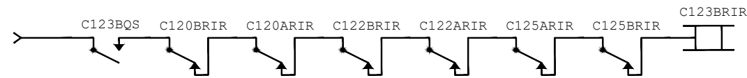
Route Initiation Circuit, Signal C123 "B" Route - to Signal C120 (Reverse Running)
