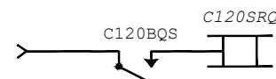
Signal C120 to Signal C123 (Straight) Route Request Indication To Central Office
