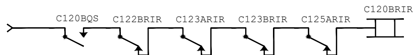
Route Initiation Circuit, Signal C120 "B" Route - to Signal C123 (Reverse Running to Eastridge)
