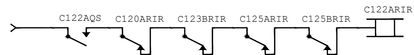
Route Initiation Circuit, Signal C122 "A" Route - to Signal C125 (Normal Running to Eastridge)
