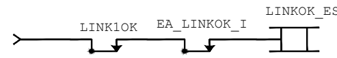
Link Health Status, Alum Rock Vital Processor to Eastridge Vital Processor "A"
