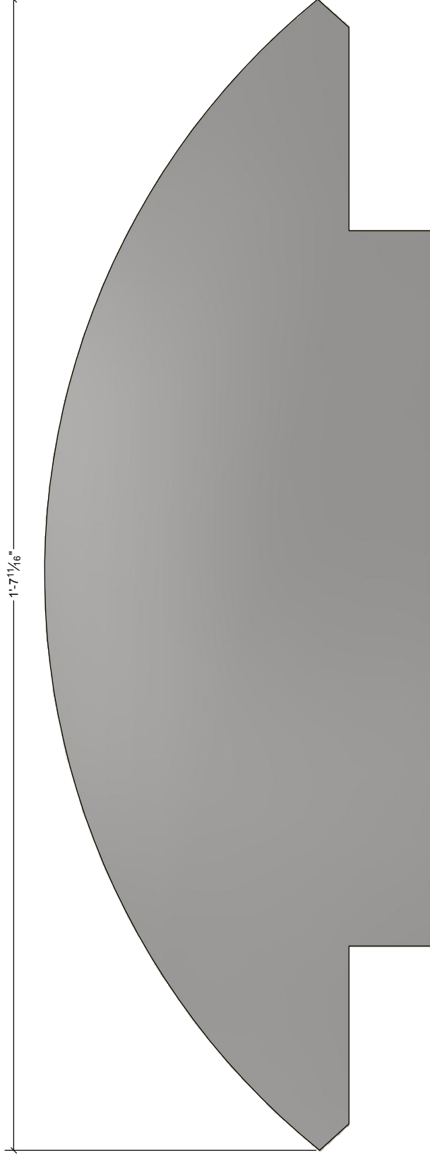
STIFFENER L7 - PLAN VIEW SCALE 8"=1'
