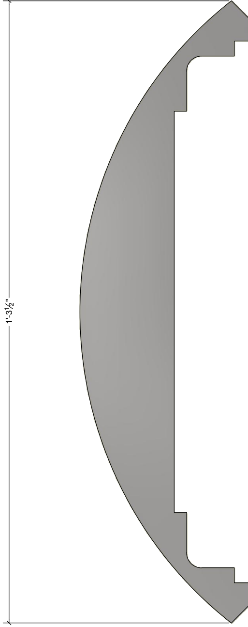
REAR STIFFENER L2 - ELEVATION SCALE 8"=1'
