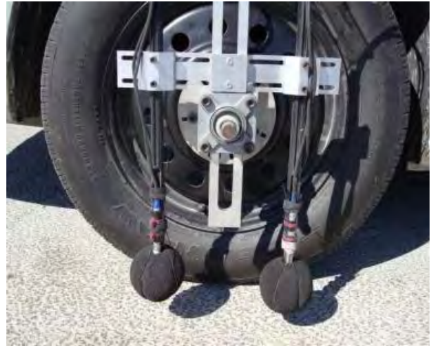
Figure 5-7: On Board Sound Intensity Measurement
