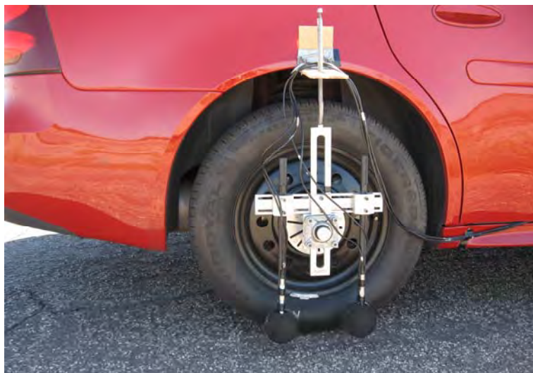
Figure 1: OBSI measurement fixture mounted on test vehicle
